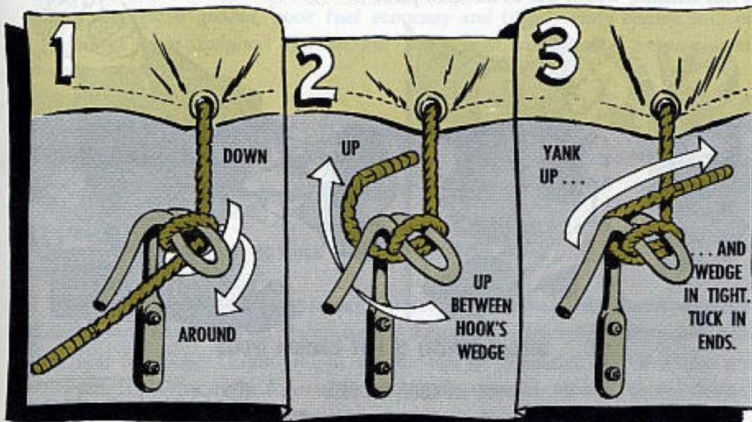
That does away with complicated sailor-type knots, and makes putting a tarp on or taking it off just a matter of a few flips. Easy to get a tarp taut over the top, too.
