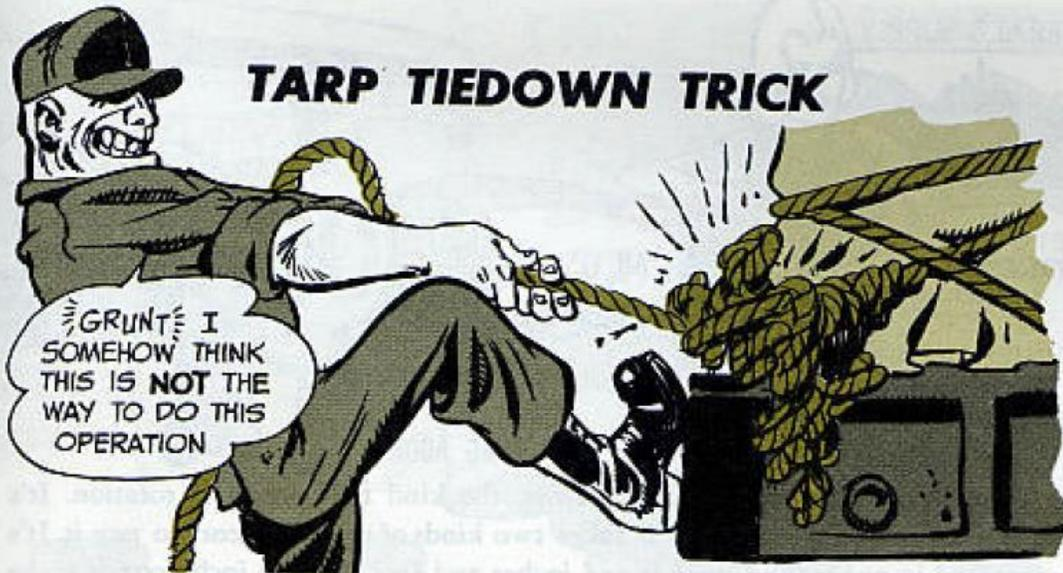
That pigtail-style wedge hook set-up on the side of your cargo truck was put there to make things easier for you—so don't try to make it tough. It's a lashing-type wedge hook (FSN 2540-706-4246).
